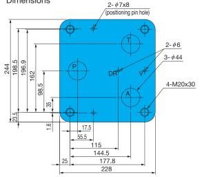
The gasket surface dimensions comply with the ISO standards shown below.
